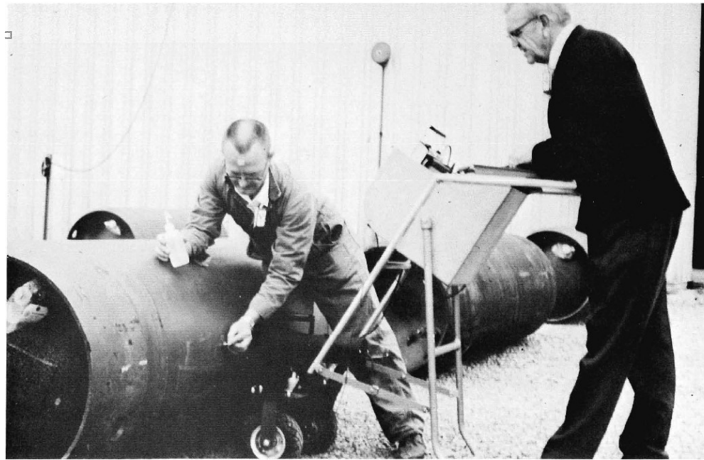
Fig. 10. Field measurement of ^{235}\text{U} enrichment of \text{UF}_6 in a 2-1/2-ton shipping container. A portable NaI detector is used to measure 186-keV ^{235}\text{U} gamma rays. A portable ultrasonic gauge is used to determine the cylinder wall thickness for the attenuation correction.
