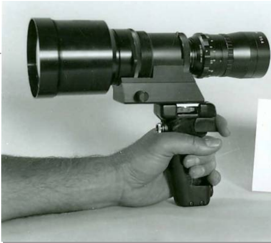
Cerenkov Viewing Device (CVD) for Spent Fuel Verification (circa 1979 )
